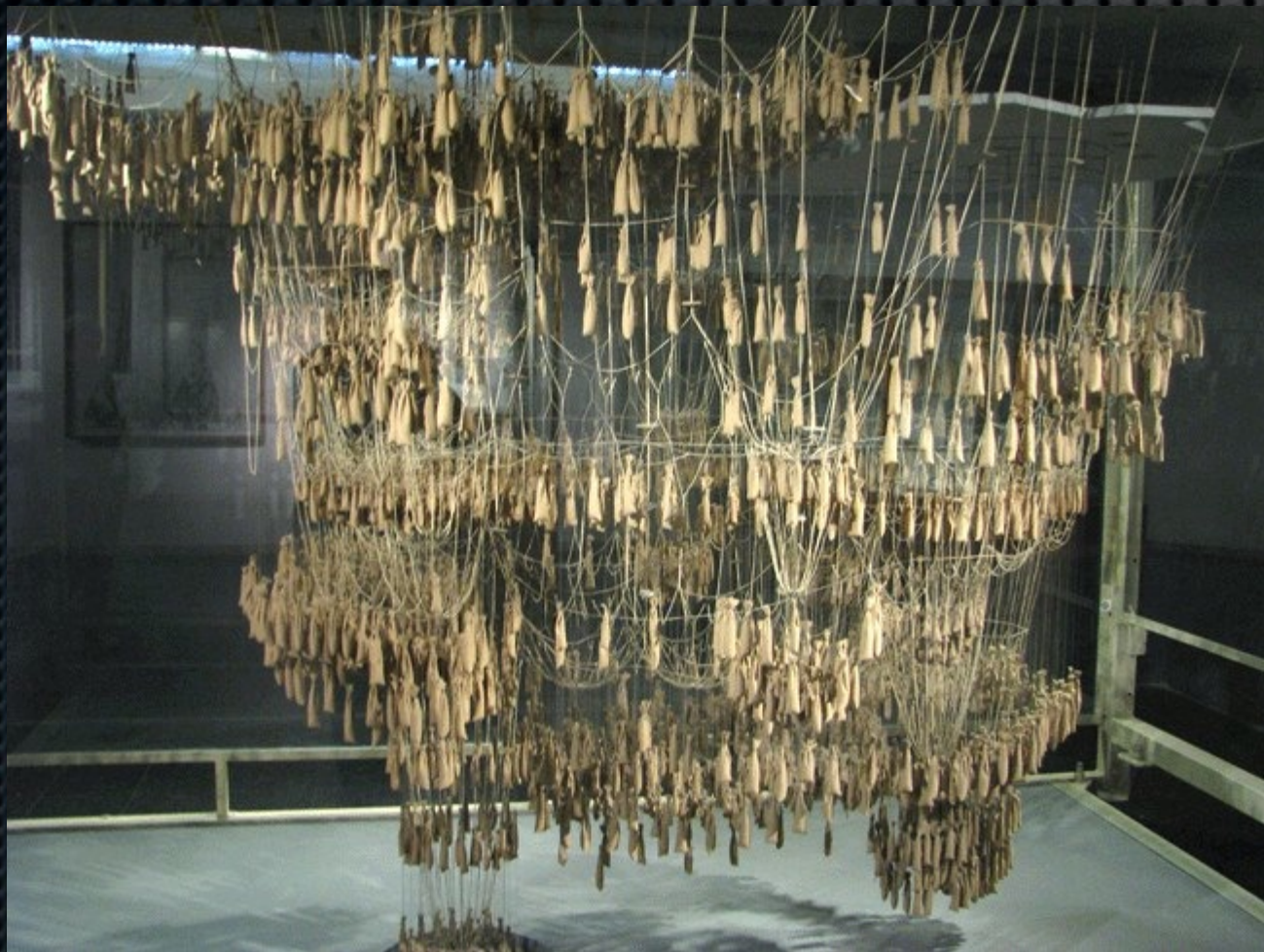
Statical model experiment A. GAUDÍ
